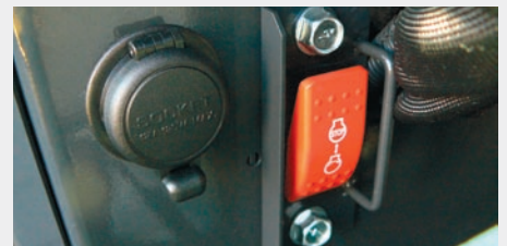
Electric engine stop (emergency stop)
